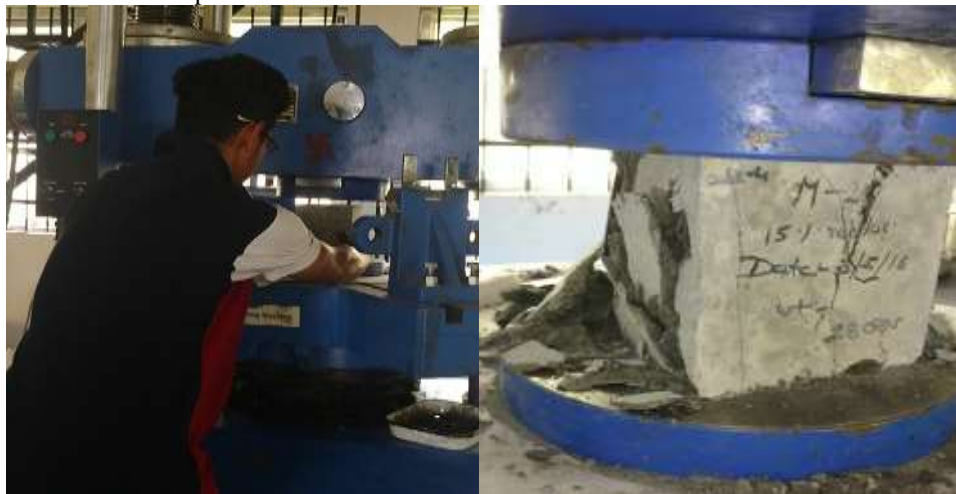
Sample tested under UTM of NITTTR lab
